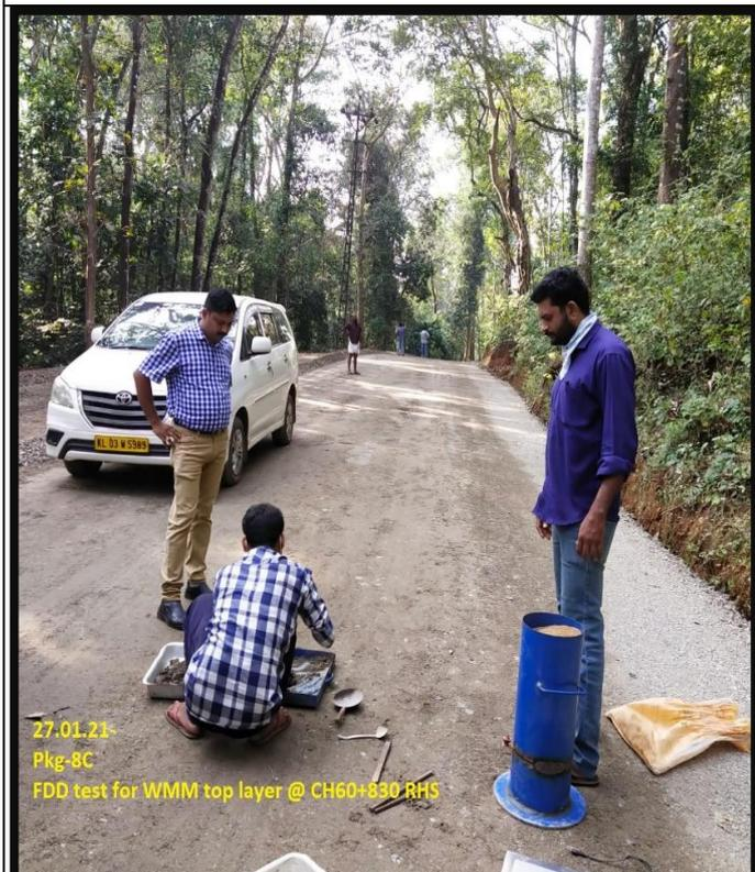
FDD Testing work in progress for WMM top layer from 60+830
