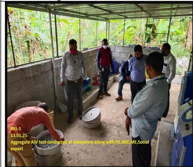
Aggregate AIV testing in progress
